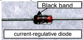
yellow is mounted in D5 when it is manufactured, but they can be replaced.
